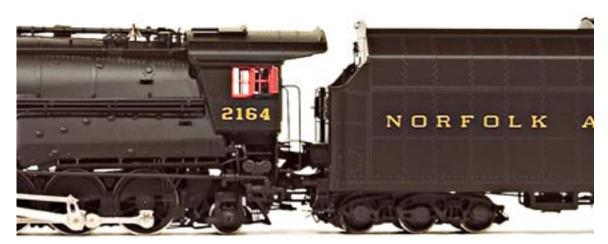
Shown above is the completed connection of the Y6a and 22C tender, notice the position of the electrical connectors.
